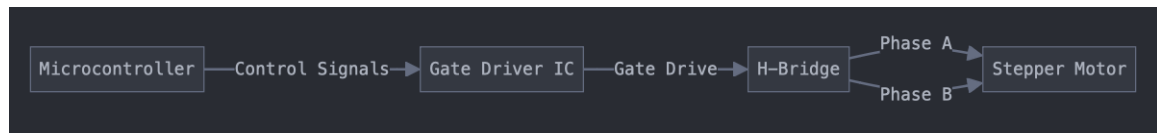
Figure 3.2.8-1 - Gate Driver Flow Diagram
